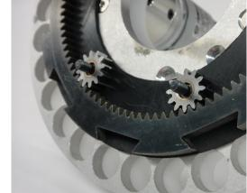
distribution gears gears are made from stock and waterjet parts. the 30 holes allow balls to travel to
