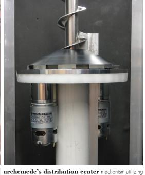
auger and motors to recirculate ball bearings
